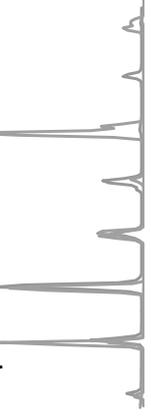
We asked three students (2 males and 1 female) to pronounce the sound of 「A」, and the aggregation rate of the frequencies was shown as a graph. Although there were some differences in frequency, N harmonics were repeated at regular intervals.
